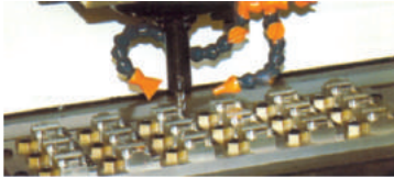
Cam action side clamping
